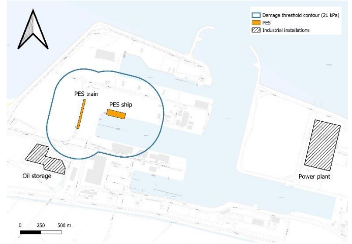
Figure 10: Pressure damage threshold contour of 21 kPa, including PES locations and potentially vulnerable sites.
